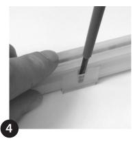
To remove KKLN-01 Lens from clip, insert a screw driver down either side of the clip. Then rock the lens against the screw driver and remove the lens.
